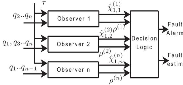
Fig. 2. GOS for an  $n$  sensor system.
