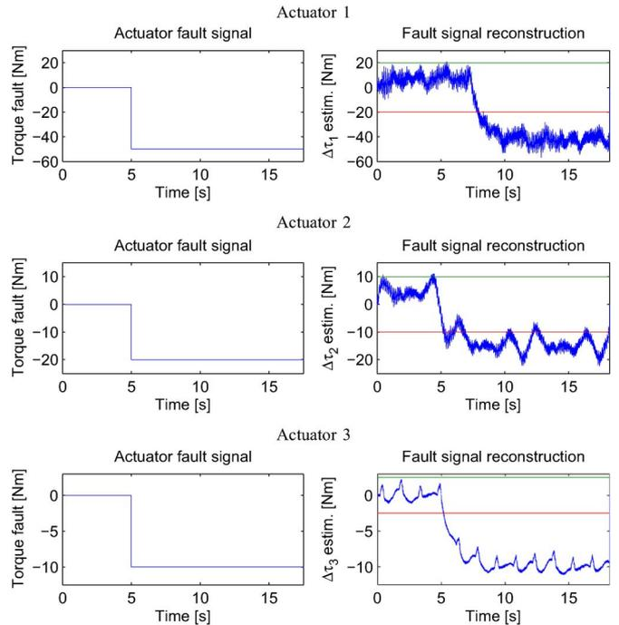
Fig. 5. FD experiment ( $\Delta\tau$ ,  $\widehat{\Delta\tau}$  signals). Suboptimal.
