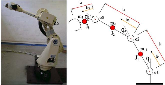
Fig. 3. SMART3-S2 robot and the three-link planar manipulator.
