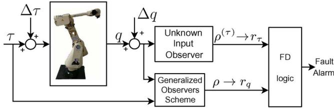
Fig. 1. Proposed FD scheme for actuator and sensor faults.
